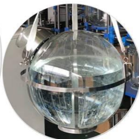
100L Evaporation Flask Hydraulic Lifting
